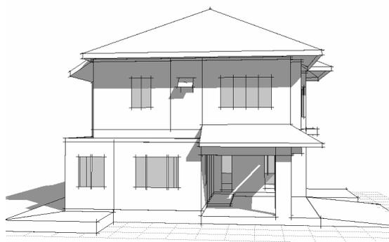
**Figure 9:** Inadequate shading on west façade of a contemporary house in the central region at 3pm in June (Source: Antarikananda, 2005)
